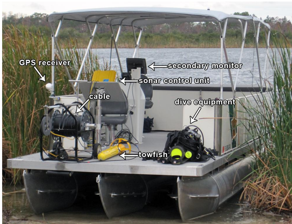
Figure 3: Pontoon boat that OCSO uses to deploy side-scan sonar with equipment labeled
