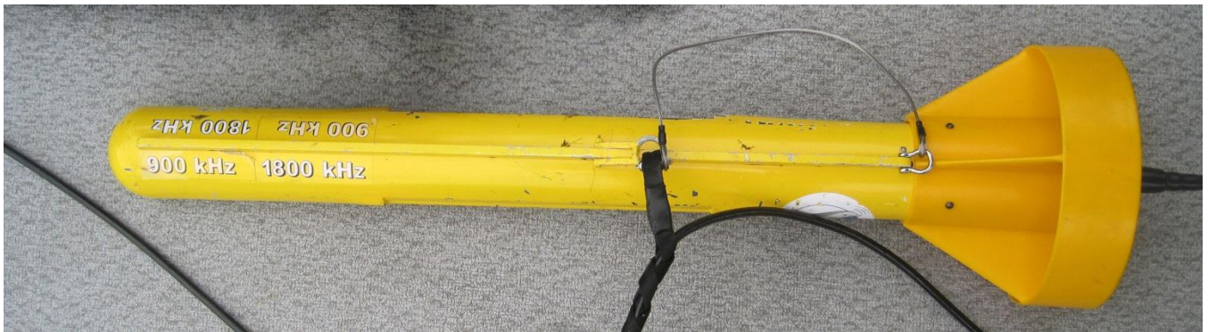
Figure 2: Centurion Sea Scan dual frequency side-scan sonar towfish
