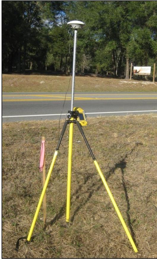
Figure 7- Point data collection using the DGPS unit at survey marker VOLV119
