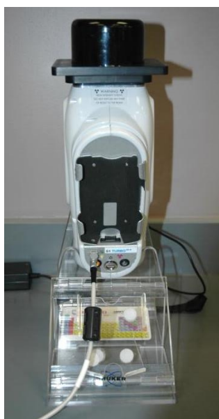
Figure 8: Bruker Elemental S1 Turbo-SDR HHXRF unit shown mounted on a vertical stand for stationary analysis.
