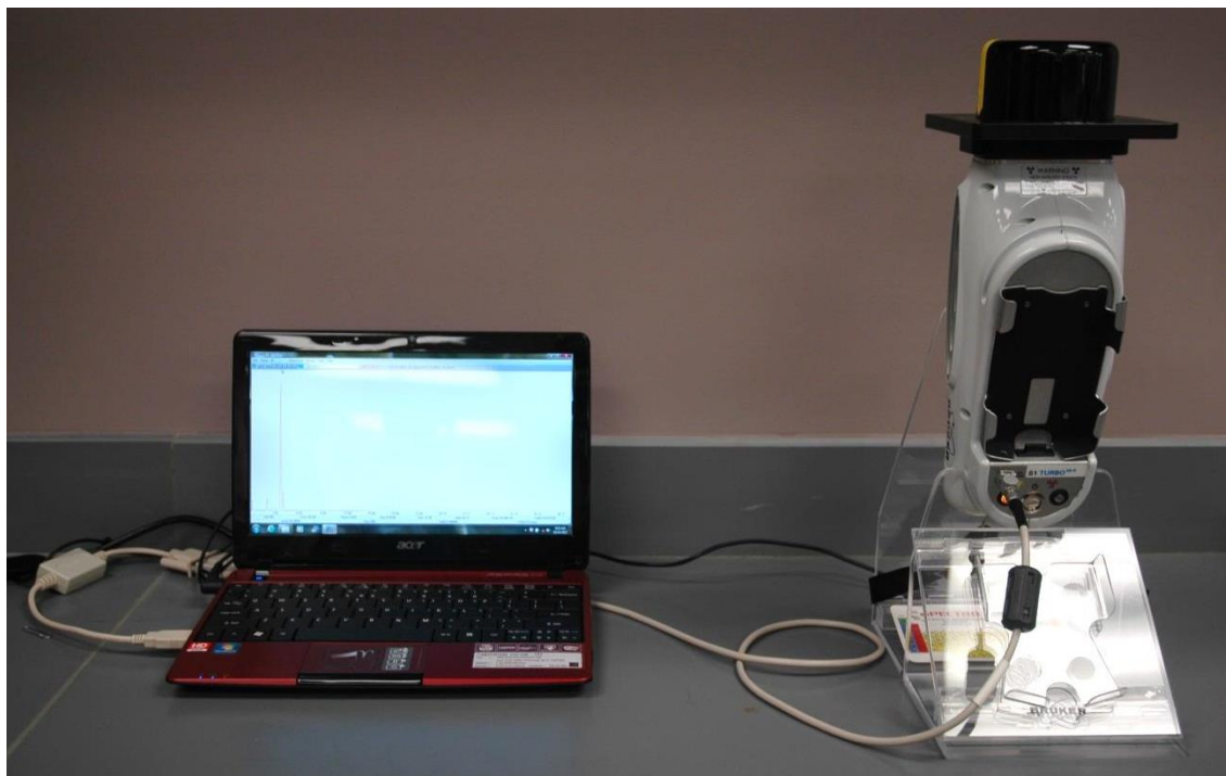
Figure 9: Accompanying laptop computer provided by the manufacturer connected to the HHXRF via the white cable in the photo. The laptop came with upgraded analytical software, SIPXRF, which was used for all data collection events and allowed for the detection of low-mass elements.
