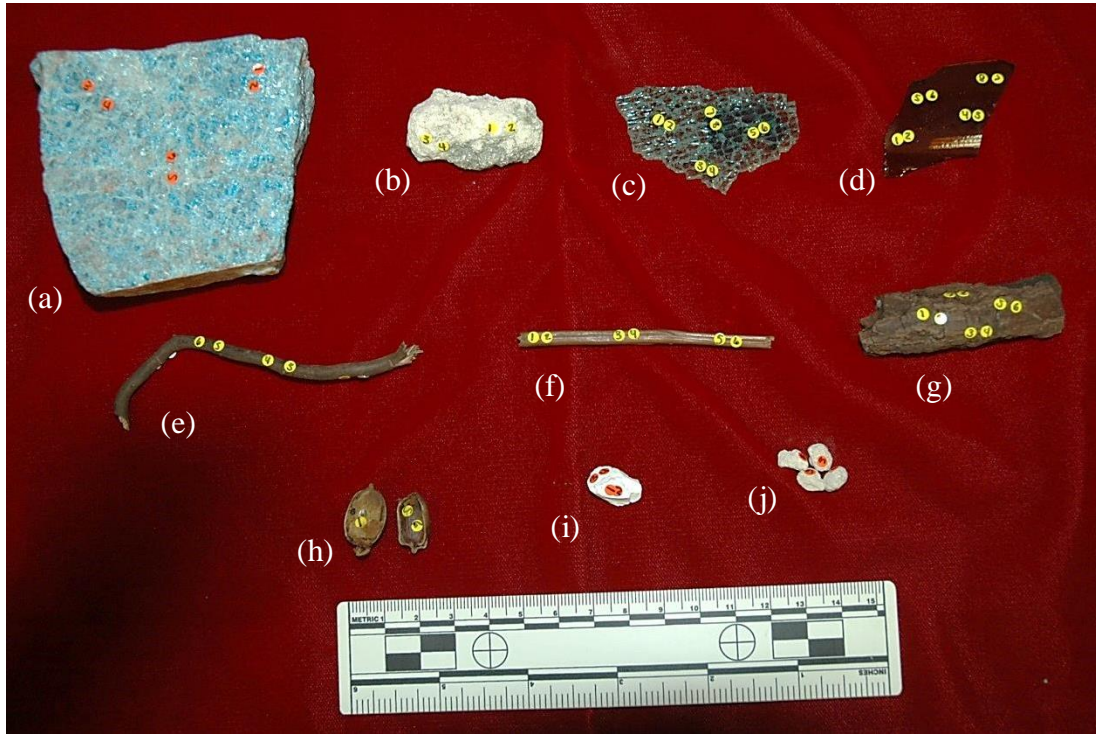
Figure 5: Non-biological materials examined in the study: (a) rock apatite, (b) limestone, (c) float glass, (d) beer bottle, (e) plant root, (f) twig, (g) bark, (h) seed, (i) synthetic hydroxyapatite and (j) rock phosphate. The stickers on the specimens denote data collection sites.
