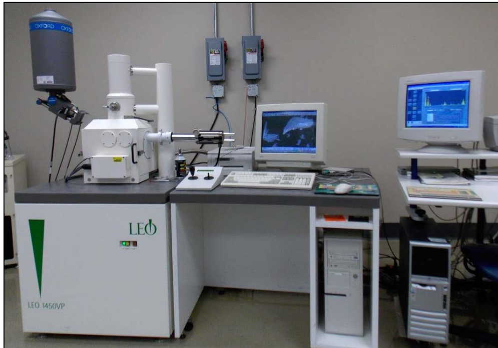
Figure 7: LEO 1450 VP Scanning Electron Microscope and Oxford Energy Dispersive Spectrometer.
