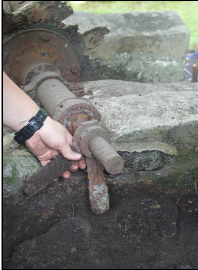
Figure 39. Pieces of gear attachment being held up to axle for context of possible attachment points.
