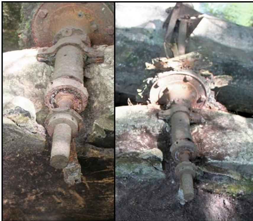
Figure 25. Portion of axle that protrudes over gear box and contains the attachment points for a potential gear.
