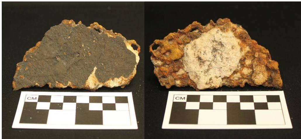
Figure 41. Example of plaster and lath material recovered in trench02A.
