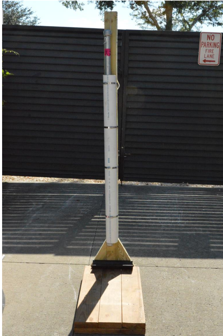
Figure 7: Custom drop apparatus modeled from Wieberg's (2006) and Shattuck's (2010) studies. A 1 ¼ - inch steel drop weight weighing 9.32kg was dropped from a height of 0.48m. A 3-inch PVC pipe acted as a guide for the drop weight. Bones were placed in the cradle at the base to ensure consistency in the point of impact
