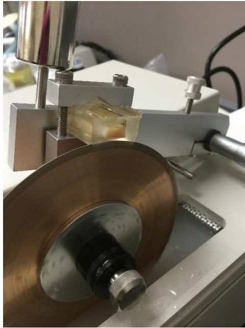
Figure 8: Thin sectioning using an IsoMet 1000 Precision Saw and a diamond wafer blade.
