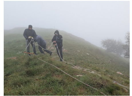
Conducting an electrical resistivity survey on a foggy, cold day in the field.
