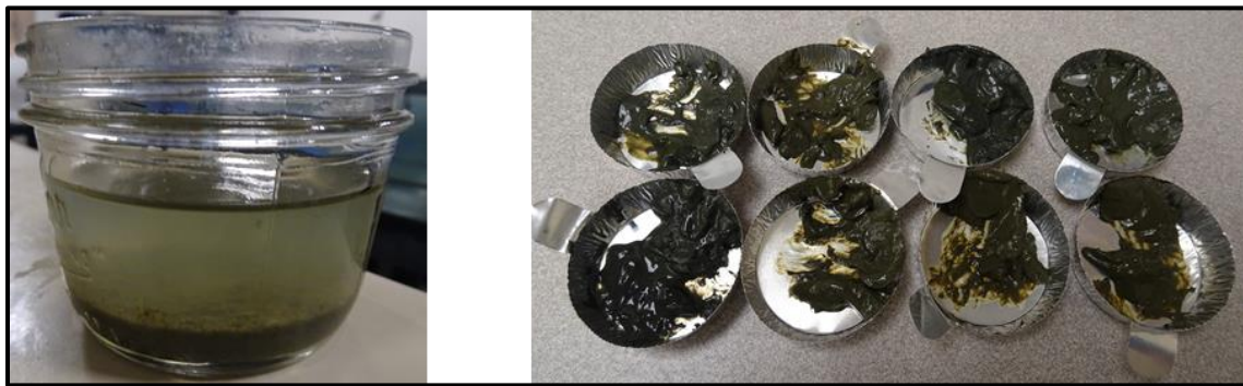
Figure 15: Left photo – example of a biodeposit sample after removal from the tank and before centrifuging to separate biodeposits from site water. Right photo – example of biodeposit color and texture after removal from centrifuge tubes and before nutrient extraction.
