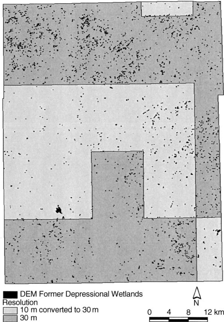
FIG. 2. DEM (Digital Elevation Model) model of former depressional wetlands within Champaign County, Illinois, USA. Delineated portions of the county include 10-m resolution converted to 30-m resolution (light gray) and 30-m resolution DEM data (dark gray).
