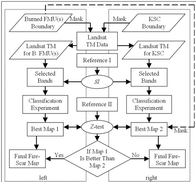
**Figure 2.** Work flow diagram of stepwise image processing for mapping fire scars at KSC-MINWR with Landsat TM data.
