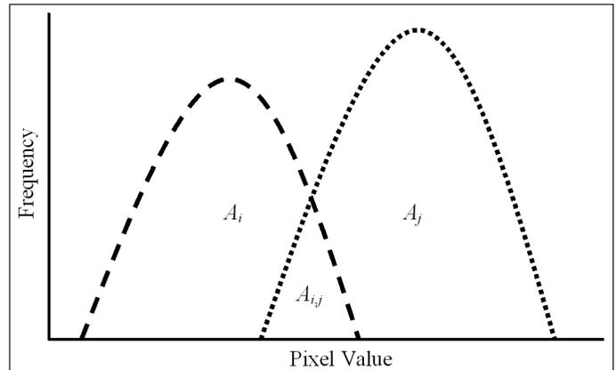
**Figure 3.** Illustration of the overlap of two histograms. Type *i* (dashed line) and type *j* (dotted line) can represent burned and unburned cover types. *A<sub>ij</sub>* represents the overlap areas between burned and unburned cover types. *A<sub>i</sub>* and *A<sub>j</sub>* represent the area for burned and unburned cover types, respectively.
