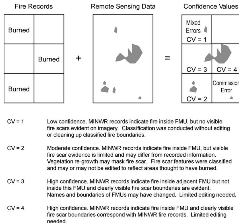
**Fig. 2.** The process of determining and labeling fire boundary confidence values (CV). The diagram on the left symbolizes the fire records kept by Merritt Island National Wildlife Refuge (MINWR). The diagram in the middle represents fire scars mapped from satellite imagery. The diagram on the right shows how the information is used to label mapped confidence values.
