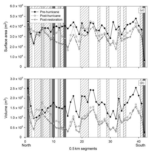
Figure 3. (a) Surface area and (b) total sand volume of each  $\sim 0.5$  km beach segment along the 21 km study area before and after the hurricanes and after restoration. Dark grey areas are 100% natural, light grey areas are <50% restored, striped areas are 50-99% restored and white areas are 100% restored. Post-hurricane and post-restoration surface area and volume measurements were both significantly different from pre-hurricane measurements (P < 0.001 in each case).
