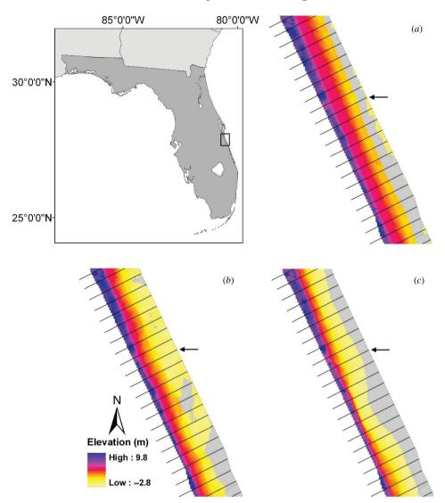
Figure 1. Map of study area and a representative  $\sim$ 500 m stretch of the ACNWR. LiDAR images show elevation changes from (a) pre-hurricane, (b) post-hurricane and (c) post-restoration. Lines show the location of the profiles, which are spaced at 25 m intervals and the black outline indicates the boundary of the St Johns River Water Management District areas classified as 'beach'. Arrows indicate the representative profile that is used as an example in figure 2.
