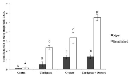
Fig. 4 Mean change in wave height after encountering shoreline stabilization treatment (±SE). Wave heights were compared using a two-way ANOVA. New=new restoration with new, clean, stabilized oyster shells and cordgrass plugs at planting densities used in Mosquito Lagoon.
