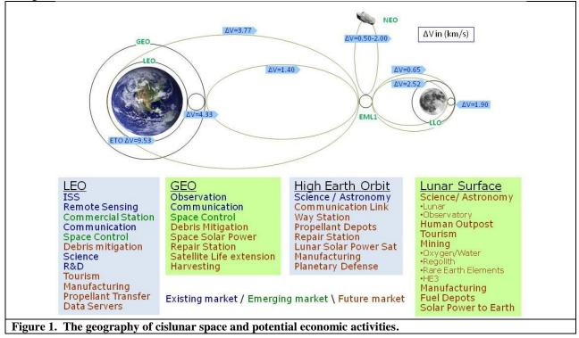
LEO consists of a region of space up to about 1000 km above the Earth's surface. Useful orbits in LEO are nearly circular and have orbital periods of around 90 minutes. A wide range of inclinations are employed. Highly
