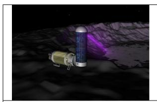
Figure 9. The Power Tower System delivered to the rim of Shackleton Crater by Vulcan XEUS. The Solar Array telescopes to 100m height to passively soak up the nearly continuous grazing sunlight. Lasers mounted to the top of the tower beam energy into the permanently shadowed crater to support the water extraction.
