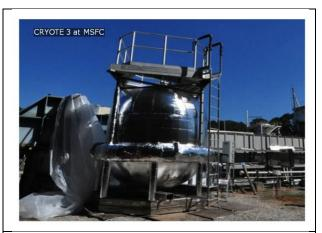
Figure 5. CRYOTE 3. A long duration cryogenic test bed.
