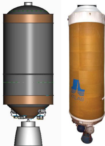
Figure 2. ACES size vs Centaur (Example Shown with BE-3 Envelope)
