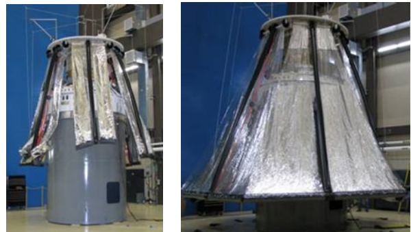
Figure 26 – ULA, ILC-Dover and NASA have developed a pneumatically deployed sun shield to support long duration cryo-storage. Courtesy ULA
