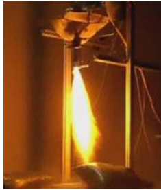
Figure 32 – Testing has demonstrated the functionality of this low cost hydrogen/oxygen thruster. Credit Innovative Engineering Solutions
