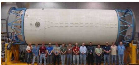
Figure 34 – Cryo-fluid testing of a Centaur tank can provide invaluable data on the actual performance of proposed thermal protection schemes. Courtesy ULA
