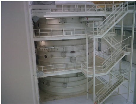
Figure 14 – NASA KSC’s O&C vacuum chamber provides the size required for system check out of the completely integrated depot prior to launch. Courtesy NASA
