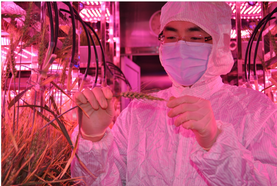
Figure 9. Dr. Chen Dong of Beihang University inspecting wheat plants inside the Lunar Palace 1 facility in Beijing, China. Note the pinkish colored light from high output red and white LEDs to grow the crops that supported three crew members for 105 days. Photo courtesy of Prof. Hong Liu, Beihang University.
