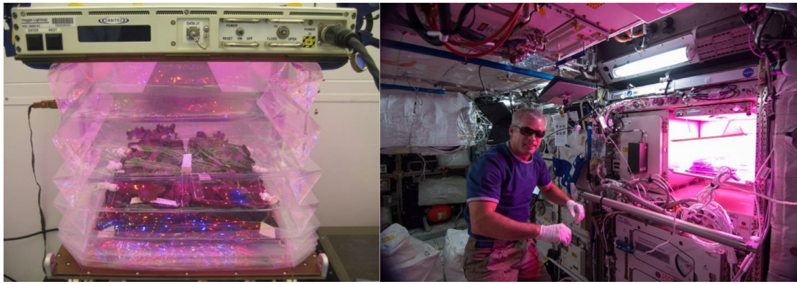
Fig. 12. VEGGIE prototype during ground tests (left); NASA astronaut Steve Swanson next to VEGGIE after the deployment on-board ISS (right) (Stromberg, 2014).
