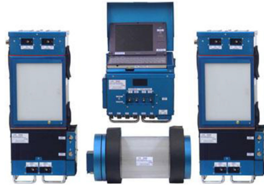
Fig. 8. Lada; control and display module (upper center), growth modules (left and right), water tank (bottom center) (Bingham et al., 2002).
