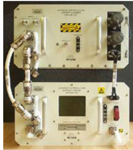
Fig. 6. Advanced Astroculture ISS plant growth chamber (Link et al., 2003).
