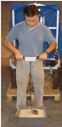
Figure 10: Measuring static penetration forces of the Surveyor-like scoop.
