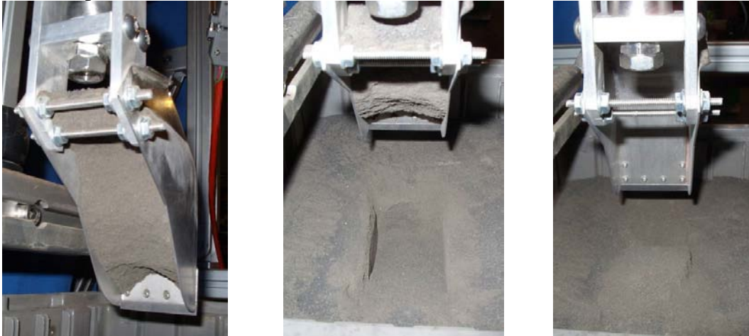
Figure 16: (Left): Material retained in the scoop due to bridging after penetration test in compacted JSC-1a. (Center): The corresponding sharp-walled cavity in the test bin. (Right): “Tapping” the scoop by running the percussor at low frequency for one or two cam rotations was an effective way to clear the retained material.
