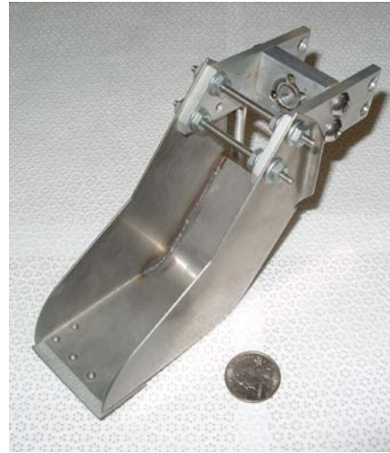
Figure 9. Surveyor-like scoop was used for excavation tests.
