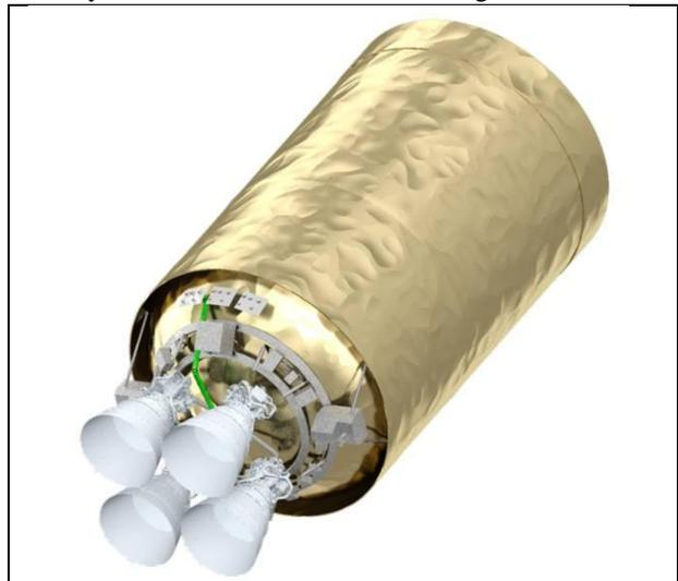
**Figure 3. Advanced Cryogenic Evolved Stage (ACES). The backbone of the cislunar transportation system.**
