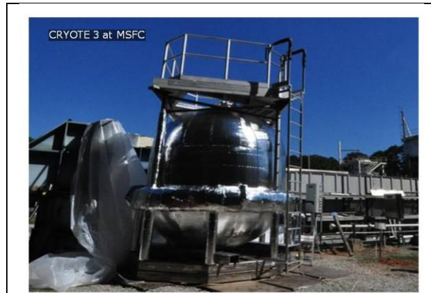
**Figure 5. CRYOTE 3. A long duration cryogenic test bed.**
