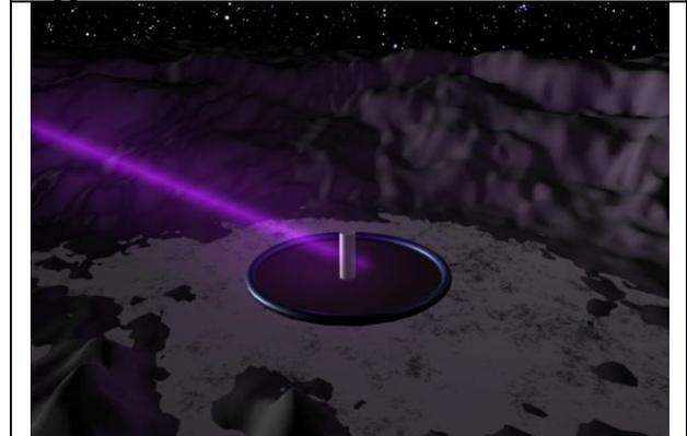
**Figure 10. The Water Extraction Facility sublimates the ice under a large engineered tarp, collects and compresses the diffuse water vapor and condenses the vapor to liquid water for storage and eventual transfer to the Water Processing Facility.**
