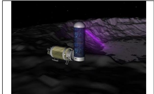
**Figure 9. The Power Tower System delivered to the rim of Shackleton Crater by Vulcan XEUS. The Solar Array telescopes to 100m height to passively soak up the nearly continuous grazing sunlight. Lasers mounted to the top of the tower beam energy into the permanently shadowed crater to support the water extraction.**
