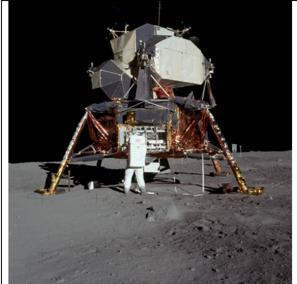
Figure 2. Apollo's Lunar Excursion Module utilizing dense, storable propellants consisted of multiple propellant tanks clustered in a compact system. Credit: NASA.
