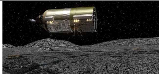
Figure 8. DTAL's provides clear surface view with minimal surface disturbance using distributed, small thrusters providing the ability for final landing location changes.
