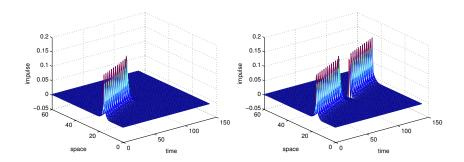
A slightly faster impulse is able to pass through the defect.
