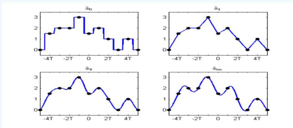
**Figure:** Cardinal spline interpolations of the discrete time signal of degree  $d = 0, 1, 2, \infty$ . The interpolations become increasingly smooth and approach the sinc interpolation as the order increases
