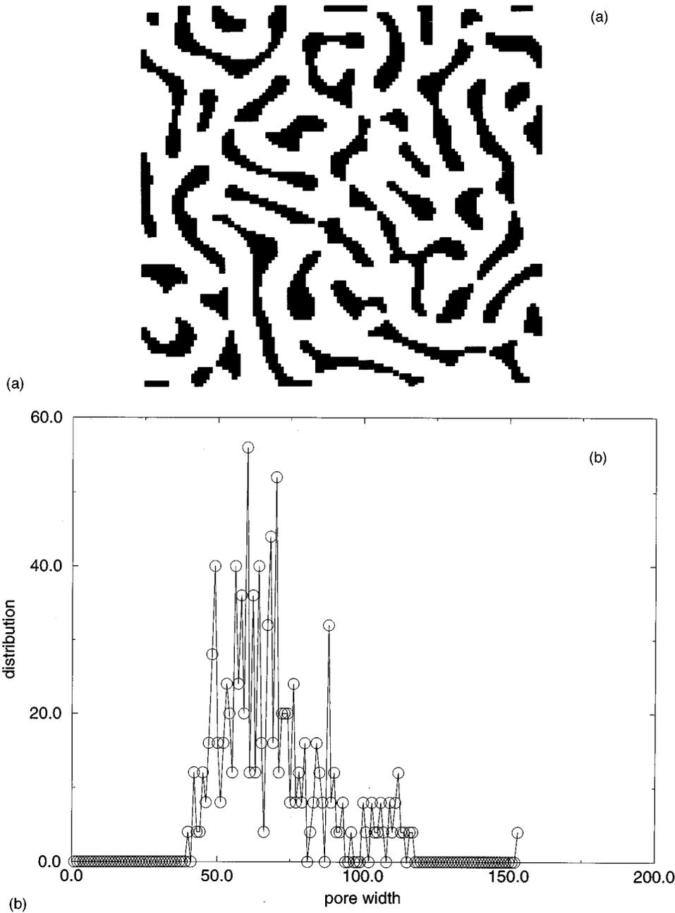
FIG. 1. (a) Picture of a typical porous media used in the simulation. The porosity is 80% and the average pore width is 68 units. The media is constructed from a square mesh of  $512 \times 512$  lattice; (b) distribution of pore sizes in the above medium.
