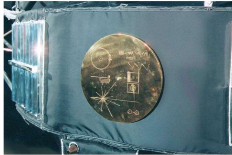
b Voyagers 1 and 2 carry a phonograph record—a 12-inch gold-plated copper disk containing music, greetings, and images from Earth.
