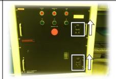
STEP 3: Turn on, in this order, the system, generator, and pump green "ON" push buttons.
