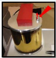
17. Open the chamber lid and remove the sample.
