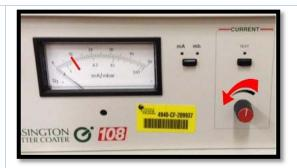
11. Turn the pressure gas control knob clockwise and set the pressure to 0.08 mbarr.
