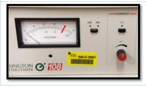
10. Turn control knob counterclockwise until the pressure gets to 0.4 mbarr. Then wait 10 seconds.
