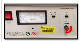
8. Turn on Sputterer by pressing the ON button on the front panel.
