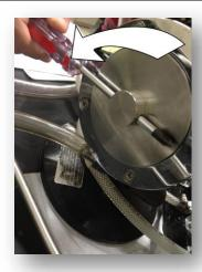
8. You should be able to see the acetone filling up the bottom half of the chamber through the viewing window.
