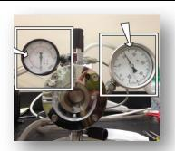
15. Gradually open the vent valve to release the chamber pressure. Opening too quickly will cause recondensation of CO<sub>2</sub>.
