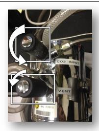
11. Leave the inlet valve fully open, and the vent valve slightly open to maintain the liquid level.
