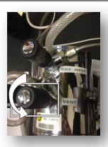
5. Unscrew the rear enclosure. You may have to use a screwdriver or Allen wrench.
