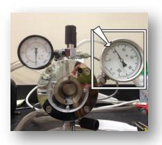
10. Open the vent valve slightly to release trapped air in the chamber, then fully open the inlet valve rapidly to fill the chamber with liquid CO<sub>2</sub>.
