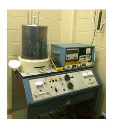
1. Vent the Chamber using the (air admittance) valve. Turn CCW. This will take 30-40 secs, until hissing stops, to vent to atmospheric pressure. Close valve after atmospheric pressure is attained.
