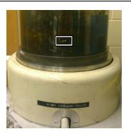
5. Replace lid and Blast Shield. Ensure that the lid is properly fitted to the seal.
