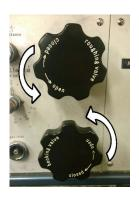
9. Wait until the chamber is pumped down to at least 80 mTorr. This will take approximately 7 mins. Refer to the data tables to ensure it is being pumped down at the proper pace.
