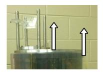
3. Remove Bell Jar by lifting approximately 1 foot from the base, and lay it on the table. Insert either rod or boat for evaporation along any other samples.
