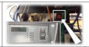
21) Open the chamber gate valve by switching up the red switch located to the right of the lower panel.
