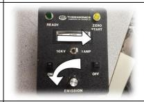
31) Momentarily press the "ON" button on the hand held controller. The "HV On" lamp should come on.
