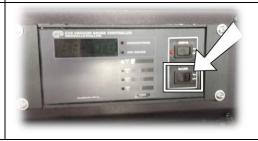
satisfy the pressure interlock of the Ebeam power supply
