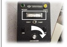
rate is achieved open the shutter and click "zero all" to start the deposition on to your sample. When the desire thickness is reached, close the shutter and very slowly ramp down the emission current so not to thermally shock the crucible liner. When the emission knob is fully counterclockwise momentarily press the OFF button on the remote. Wait approximately 2 minutes before the next step
