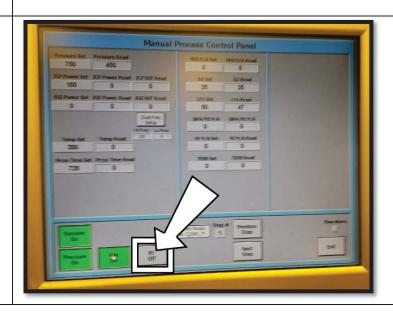
13) When the timer reaches the set time MANUALLY turn off the RF by clicking the green "RF on" button.
