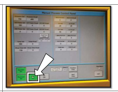
11) After pressure and gases stabilizes around their set point, turn the RF on
