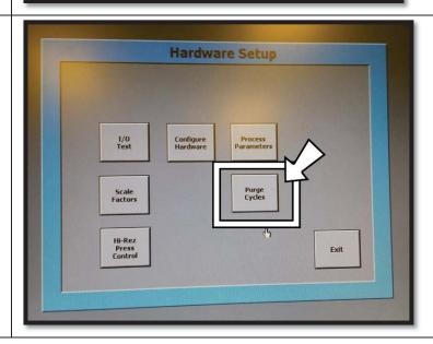
9) Switch chamber purge to "No" (square should be gray NOT GREEN). Exit Purge Cycle Control and exit Hardware Setup
