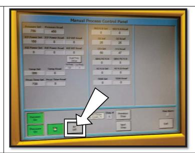
14) Click the gas button to turn the gases off DO NOT hit the Pressure or Vacuum buttons
