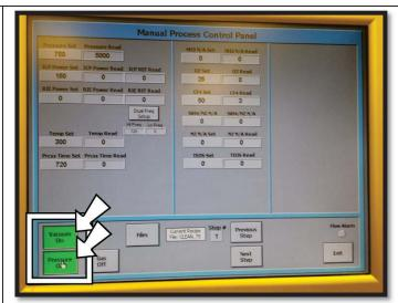
8) Wait until the pressure read in the top left of the screen is less than 100
