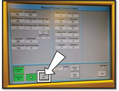
12) When the Timer reaches the set time and the process is finished, turn the RF off MANUALLY by clicking the green "RF on" button.
