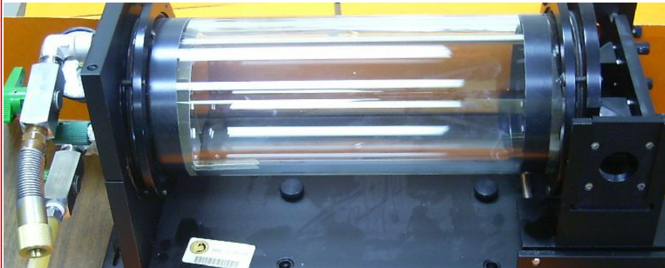
Fig. 1. Multipass 10 m White cell. Input and output are via turning mirrors and vacuum windows on the right. Internal mirrors are evident on the left. The entire system was heated using a copper shroud.
