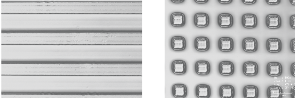
Fig. 2: Optical microscope images of 1-dimensional and 2-dimensional gold gratings.
