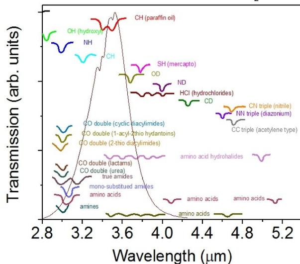
Above graph represents spectra of molecules in the range of 3.4 μm LED, superimposed on the measured spectrum of IR LED.
