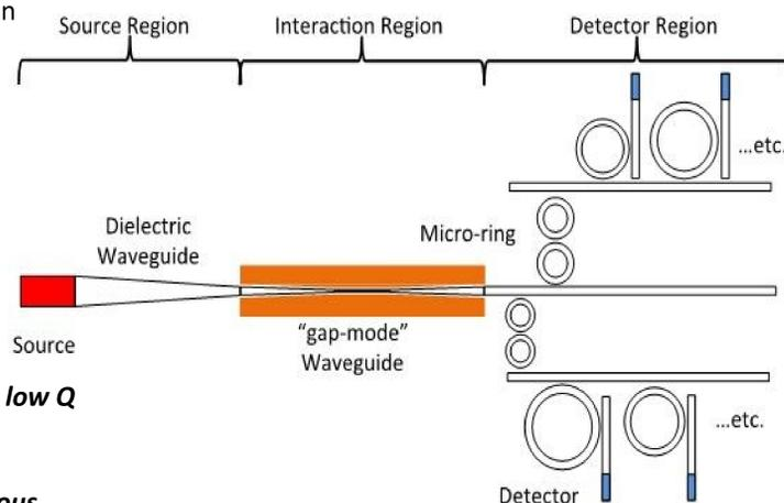
**NOTE:** Cascade ring resonators feature *low Q* and *high FRS* rings followed by *high Q* and *low FSR* rings to obtain high resolution information with *unambiguous* wavelength identification
