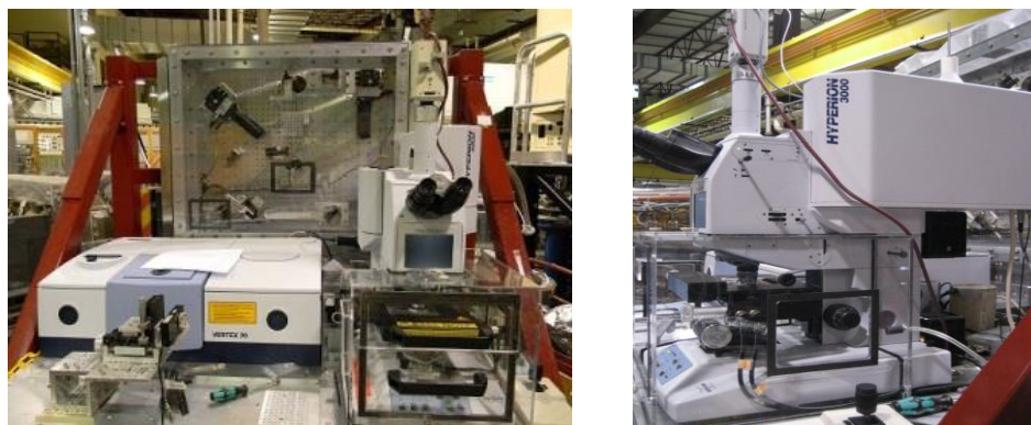
Figure 4: Experimental setup and instruments at the Synchrotron Radiation Center. Left: Optics, spectrometer, and the microscope. Right: Microscope with a joystick controlled sample stage.
