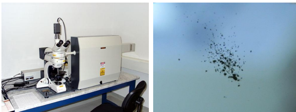
Figure 1: Micro-Raman spectrometer at Material Characterization Facility of UCF (left) and meteorite powder on a silicon substrate (right) for measurements.
