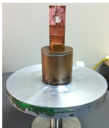
Fig. 5. (left) Photograph of the liquid nitrogen cryostat with copper-tape masking the cold-finger aperture. (right) Photograph of sample mounted on the cold finger of closed cycle cooler.
