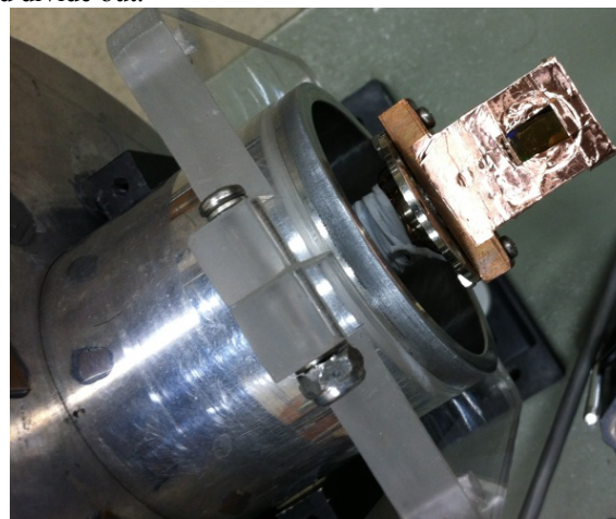
Fig. 5. (left) Photograph of the liquid nitrogen cryostat with copper-tape masking the cold-finger aperture. (right) Photograph of sample mounted on the cold finger of closed cycle cooler.
