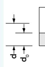
Top: Suppose a fraction (f) of a pellet has no mineral & has an area S < S<sub>0</sub> with d>d<sub>0</sub>. Then f = 1-S/S<sub>0</sub> so that EQ5 is valid. Solving for  $\alpha$  and noting  $S_0d_0 = Sd$ , EQ4 is obtained.
