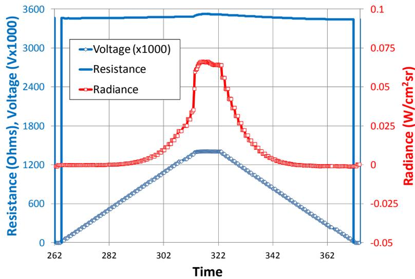
Fig. 5. Single ramp cycle of simplified test pixel
