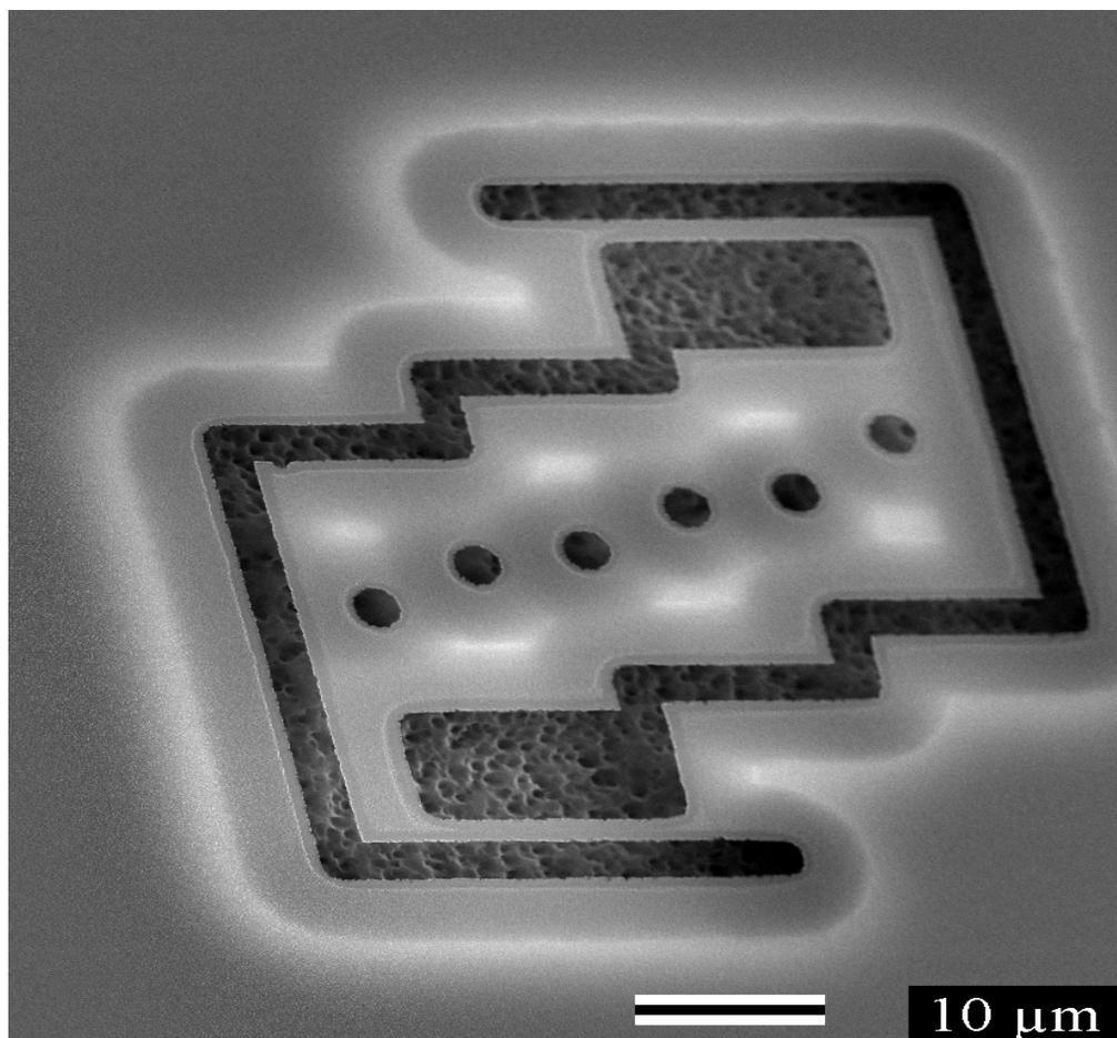
Fig. 4. SEM image of a pixel shaped test pattern from early process optimization. Here the bridge is nearly fully undercut.
