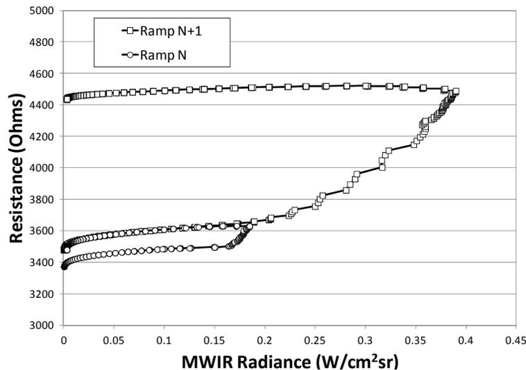
Fig. 6. Pixel resistance vs. average radiance for 2 heating cycles.
