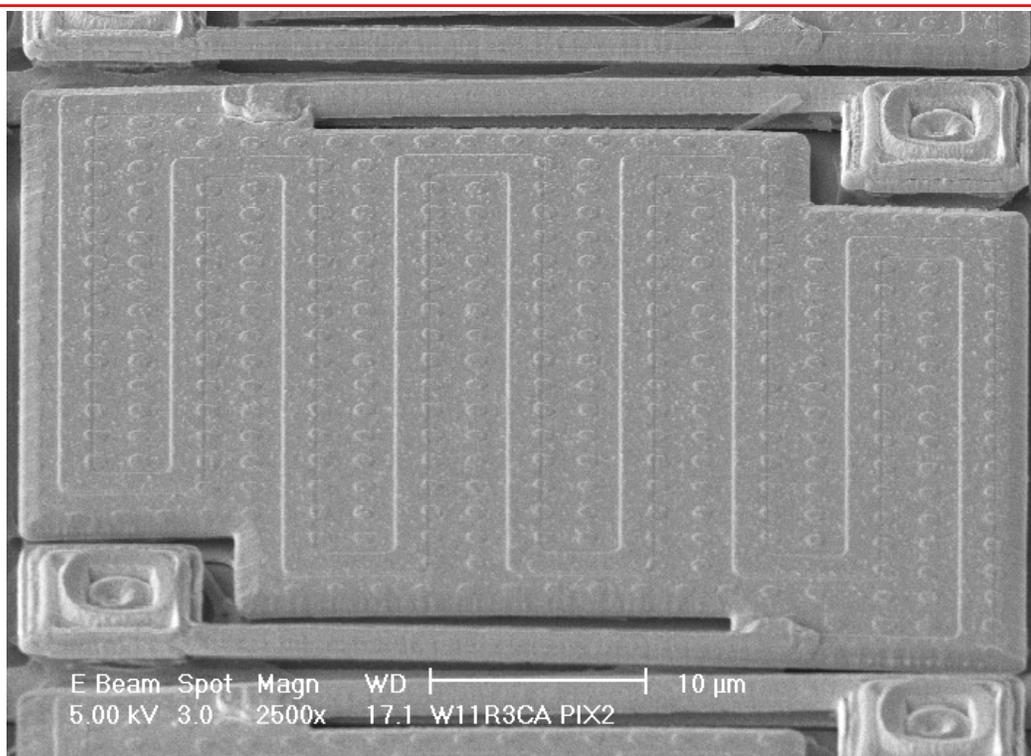
Fig. 1. Example pixel from infrared scene projector array.
