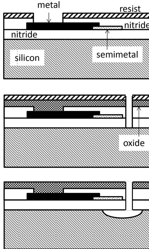
Fig. 2. Schematic illustrations of fabrication process. (Top) pad exposure etch, (middle) outline etch, (bottom), undercut etch.
