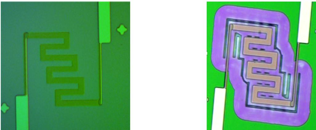
Fig. 3. Optical microscope images of pixels. The left image shows the leg and resistor traces embedded in nitride prior to processing. The right image shows a finished pixel.
