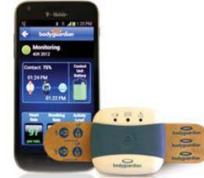
Preventice's smart bandage constantly tracks cardiac EKG and rhythm monitoring
